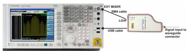
The spectrum analyzer performs an LO alignment using a detector in the mixer to set the LO Power. During the alignment the yellow Busy LED turns on. Once the alignment completes, the mixer is ready to make calibrated measurements since the conversion loss values stored in the mixer are automatically loaded to the signal analyzer.
